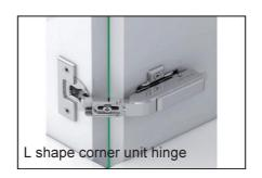
The L shape corner unit hinge backplate attaches to the adjacent door in the same way as it would attach to a cabinet, in that the fixing holes are 37mm back from the edge of the door. Please refer to our guide 'How To Fit Hinges' for further information
