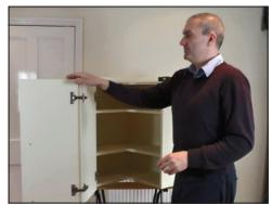
The way that this option works is that one door is attached to the cabinet with 165 degree hinges and the second door is fixed to the first door with an L shape corner unit hinge.
